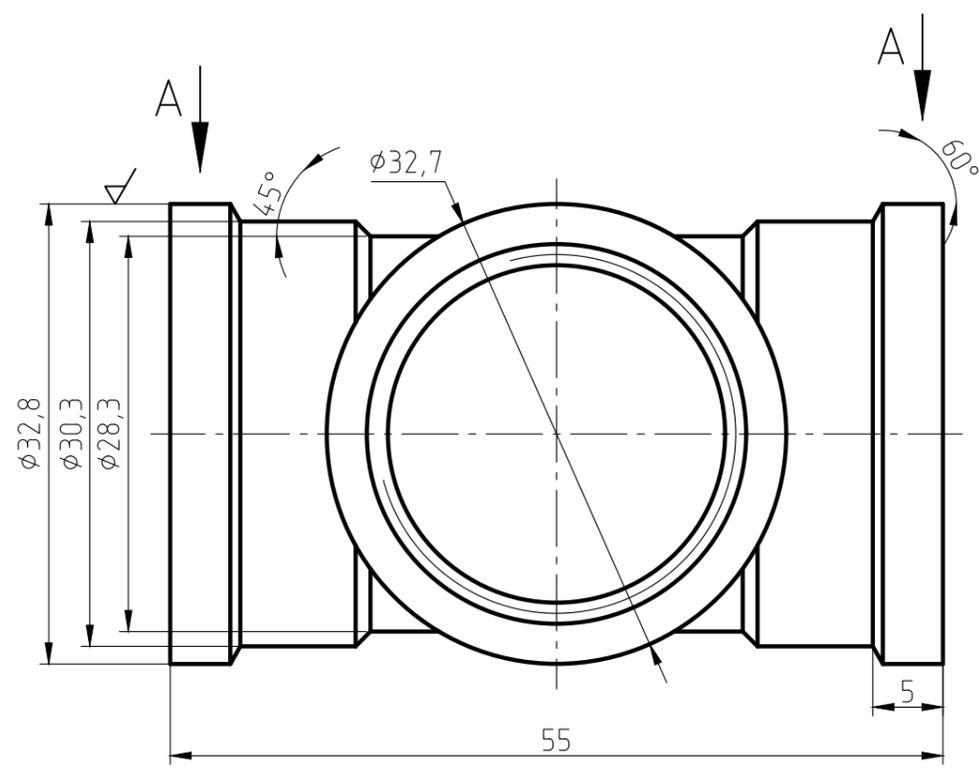
1. The parts should be 59-1 materials, no fissures surface sand-throwing treatment and nickel plating. All nickel plating.
